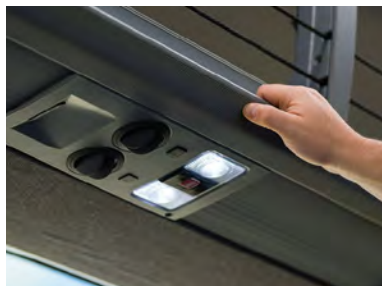
Adjustable passenger modules with LED integrated seatbelt signs.
