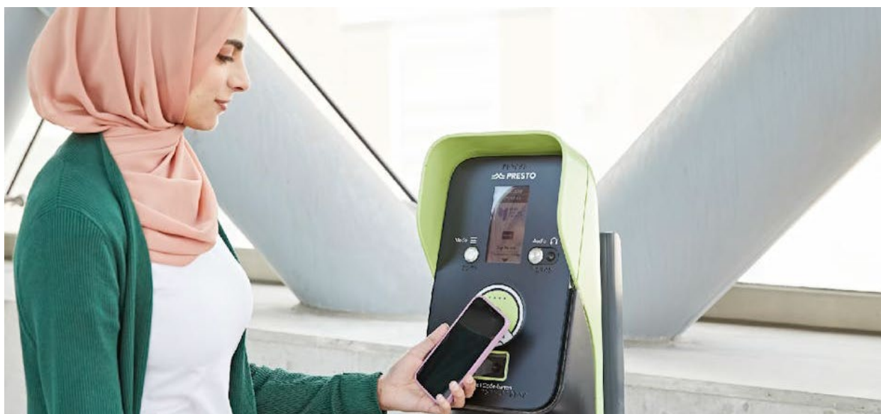
Figure 3: Contactless Open Payment Using a Phone-based Digital Wallet on PRESTO
