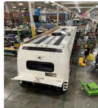
Rooftop assembly complete, batteries are in
